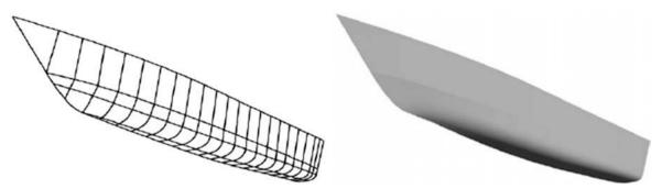
Figure 7 – Grid definition and resulting bull form for catamaran vessel
