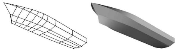
**Figure 8** – Grid definition and resulting hull form for mono-hull vessel
